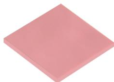
TP600 is a high thermal conductivity material with high conformability at low pressure. It is self-adhesive on both sides. When assembled with electronic components, it exhibits lower thermal resistance and better electrical insulation characteristics under low compression force. It can work stably at -40°C~150°C and meet the flame retardant rating requirements of UL94 V0.
